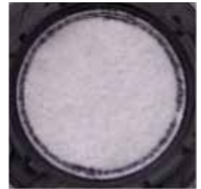
Ultrasonic welded TEM membrane with non-woven support mounted to PP based housing material.
