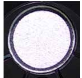
Heat welded TEM membrane with non-woven support mounted to POM based housing material.
